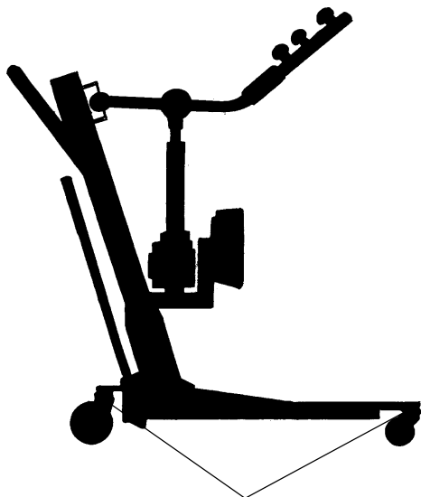
Lubricate the Bearings in the Caster Swivels
